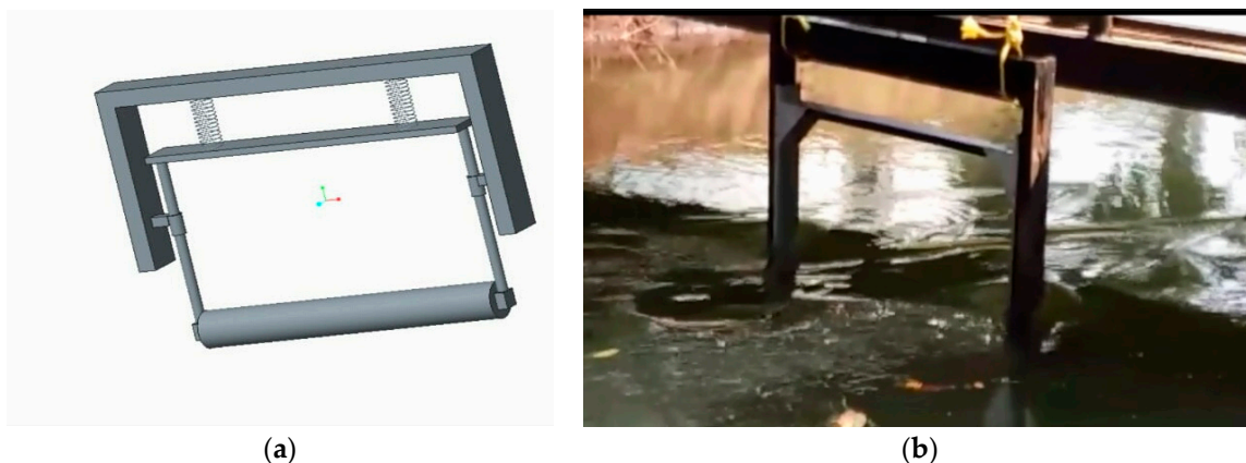
Figure 13. (a) Model of HVPG; (b) field test at Palissery irrigation canal for m^* = 0.66 and U_r = 4, 8, and 12.
